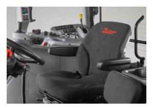
The tractor can be equipped with the mechanically or air suspended swivel seat that guarantees driver comfort.
